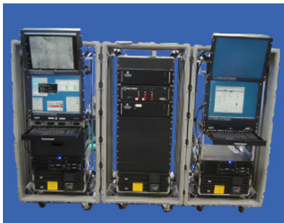
The Expeditionary Ground Control Station for the Viking 400 UAS is modular in design and adaptable to a variety of different shelters.
